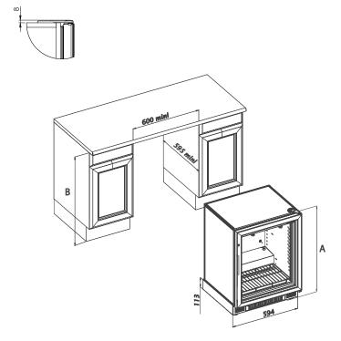
**259:** It is essential that the unit inside which the cabinet will be fitted has an opening at the top, at the back, measuring at least 540mm in length and 50mm in width (see technical door diagram).
