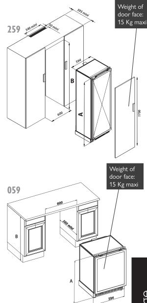
**259:** It is essential that the unit inside which the cabinet will be fitted has an opening at the top, at the back, measuring at least 540mm in length and 50mm in width (see technical door diagram).
