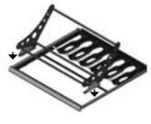
To check installation, pull the shelf forwards, the cradle should be guided in the sliders.
