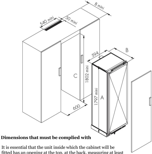
fitted has an opening at the top, at the back, measuring at least 540mm in length and 50mm in diagram).
