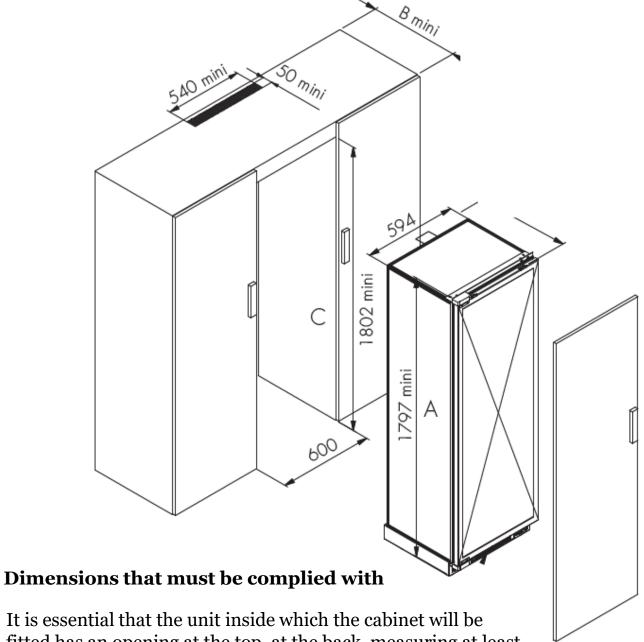
It is essential that the unit inside which the cabinet will be fitted has an opening at the top, at the back, measuring at least 540mm in length and 50mm in diagram).
